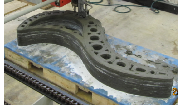
Fig. 16. The bench being printed
